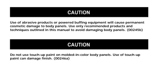
The body panels feature molded-in-color technology. The color pigment is mixed in with the material when the part is made, not applied over the surface. Molded-in-color panels require different maintenance than painted surfaces to maintain their original shine. Using methods that work on painted surfaces may ruin the finish of molded-in-color parts.
