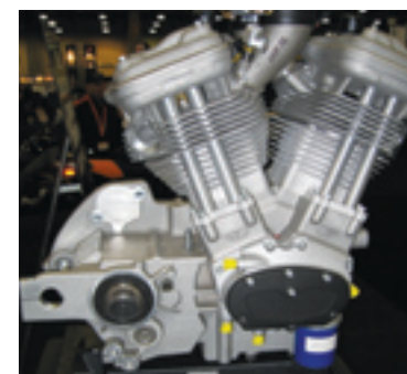
(Left) Taking advantage of the AMA Formula Xtreme rule that allows unlimited modifications for air-cooled V-twin engines, the crankcases on the engine have been recast, with a large stud pattern and a higher deck height, to make room for the bigger bores (4.08 inches).
