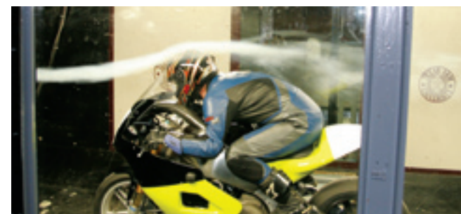
(Above) Extensive wind tunnel testing helped shape the redesigned race fairing, which resulted in 20 percent less drag and a 10-12 mph increase in top speed over the previous design.
