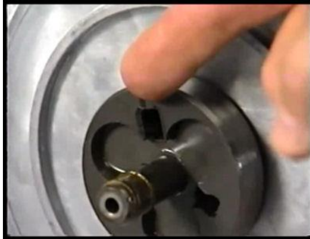
A Pin Drive unit can be identified by the Forced Air Ventilation System
