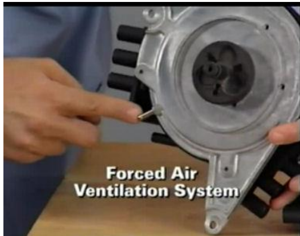
A Pin Drive unit can be identified by the Forced Air Ventilation System
