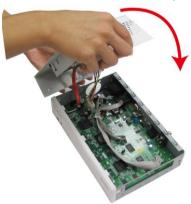
the cover back to the DVR unit and be carefully the hard disk that inside the cover.
