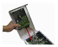
5. Hold the cover and connect the power cable 6. And then, turn the cover over carefully.
