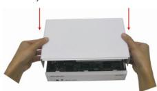
7. Hold the cover parallel with DVR unit and put 8. Finally, Push the cover forward and secure the cover
